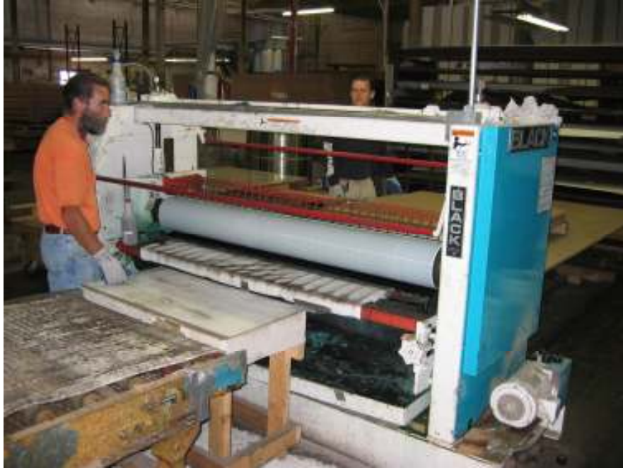
Adhesive is applied to the facing and core
